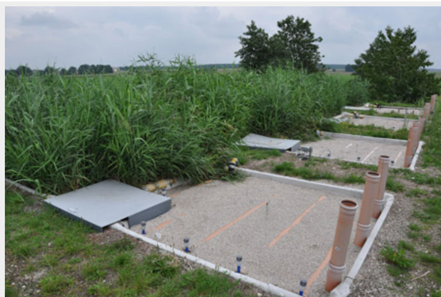
Planted and unplanted vertical flow wetlands at Langenreichenbach
